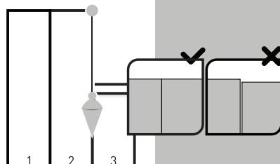
Apply the inside of the fabric to the wall in the direction of unravelling, making sure it is perpendicular. If the paper is not applied perfectly, remove and reposition it. Bring the sections together making sure the design has continuity and press lightly with a plastic spatula from the centre towards the upper and lower ends, eliminating any air bubbles and ensuring correct adherence. Immediately remove any excess adhesive and trim with a blade.
