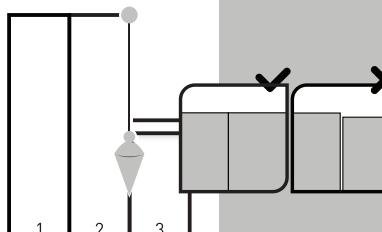
Apply the inside of the fabric to the wall in the direction of unravelling, making sure it is perpendicular. If the paper is not applied perfectly, remove and reposition it. Bring the sections together making sure the design has continuity and press lightly with a plastic spatula from the centre towards the upper and lower ends, eliminating any air bubbles and ensuring correct adherence. Immediately remove any excess adhesive and trim with a blade.
